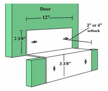
The setback is measured from the back of the door to the back of the toekick.
