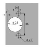
Distance D = 4mm - door offset (recommended door offset equals 1mm)
