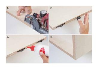
The Tenso P-14 is a self-clamping fitting with three functions: alignment, clamping and connecting. The high clamping force allows work pieces to be glued without clamps or pressure. Anchors the work piece in just seconds, without tools.
