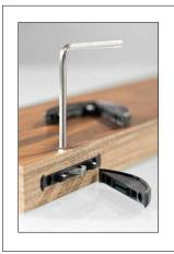
Slide Connectors into pre-cut slot, match up panels with built-in alignment tabs, lock cam lever by a turn of hex key.
