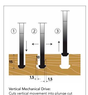
allowing installation of Clamex connectors
