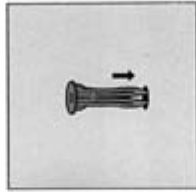
2. Insert anchor in 5/16" hole and tap flush with wall.
