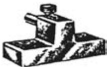
ML2 - Pin Type Lock No Key Needed.
