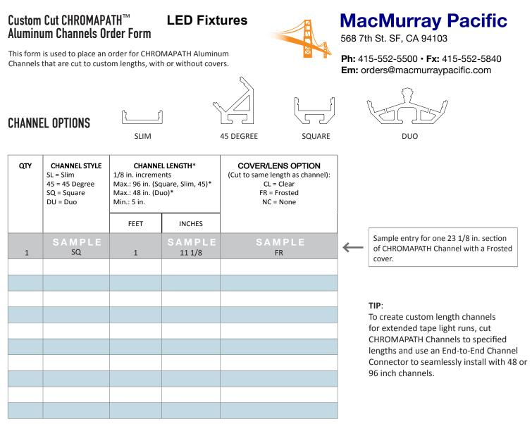
\* Length entered does not include end cap length. Each end cap adds 1/8 in. to the total channel length. End caps are sold separately.
