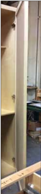
J95 Thick Door Inset Hinges used on 31" W x 93" H door.
